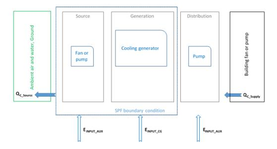
Figure 1 Illustration of SPF boundary conditions for cooling generator using standard SPF and district cooling (and other large cooling systems using measured SPF), where  $E_{INPUT\_AUX}$  is the energy input to fan and/or pump and  $E_{INPUT\_CG}$  the energy input to the cooling generator
